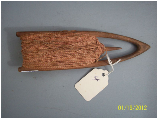
Shuttle with thread The shuttle is what holds the threads as they go between the warp threads on a loom.
