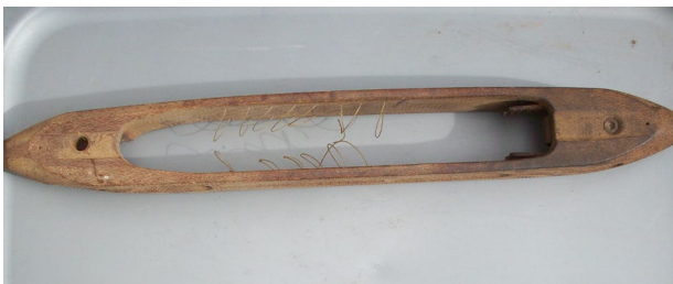
Large Shuttle This is what carries the yarn through in a large loom. A spool of thread would have been placed in the center section
